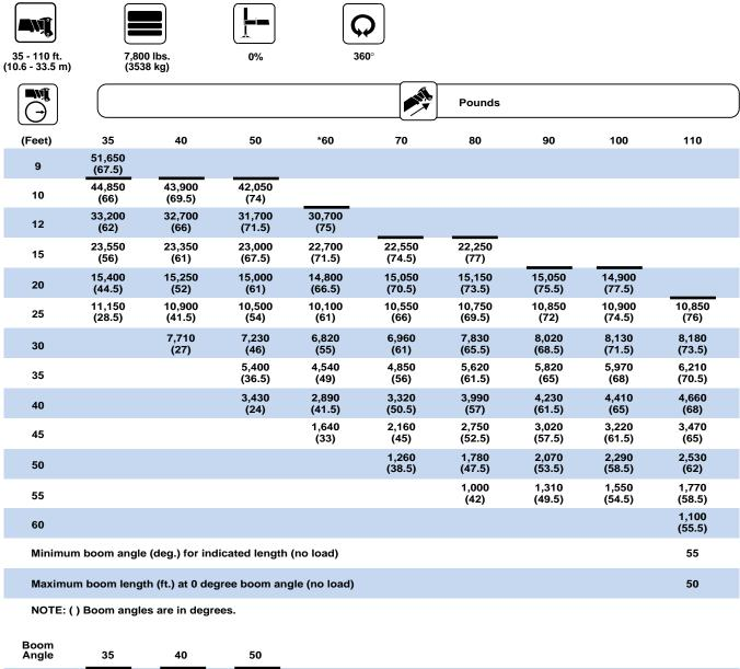
\*60 ft. boom length is with inner-mid extended and outer-mid & fly retracted.
