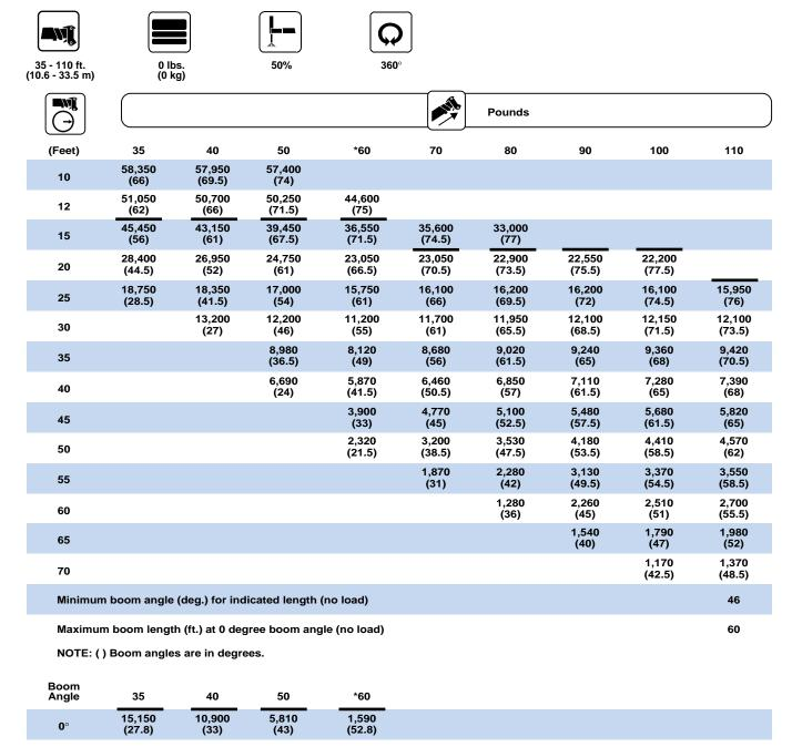
\*60 ft. boom length is with inner-mid extended and outer-mid & fly retracted.
