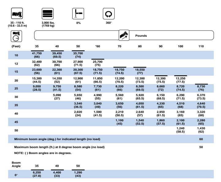
\*60 ft. boom length is with inner-mid extended and outer-mid & fly retracted.
